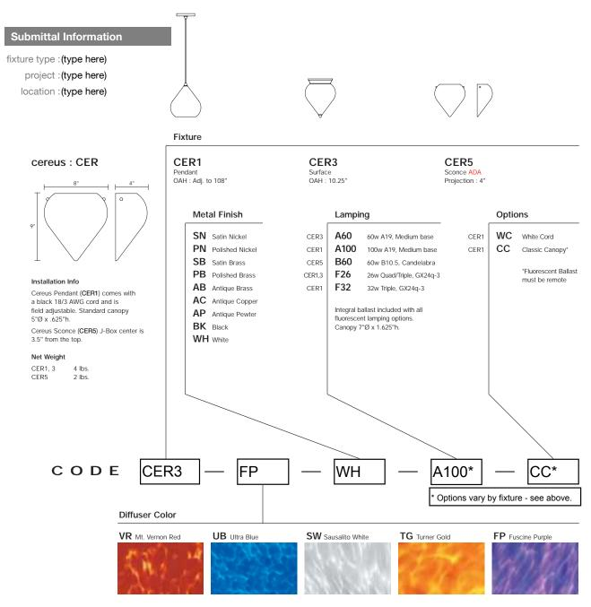
Custom glass colors, metal finishes, stem lengths, dimming ballasts, 277v ballasts, portable and track configurations are also available. Translite Sonoma has extensive custom capability. Please consult local representative or factory for details. Unless otherwise specified, standard fixture configuration is satin nickel, modern canopy and incandescent lamping. All ballasts are high power factor electronic. UL and ULC listed for dry and damp locations.
